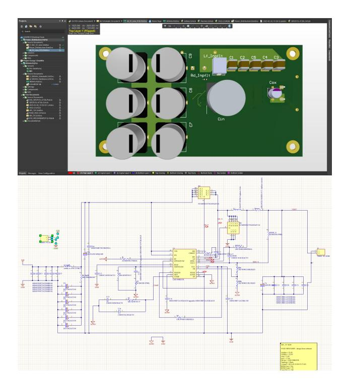
A 48V to 5V DC-DC buck converter for up to 5V, 17A to power small computers and communication on a rover for SOMTECH's URC. Design made using Altium software.
